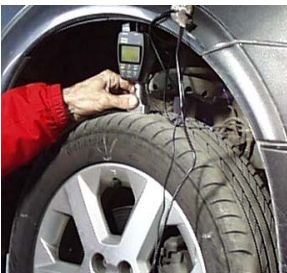
Tyre edge wear measurement
